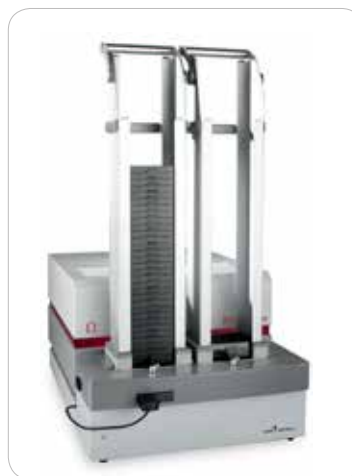
Automated microplate handling with Stacker.
